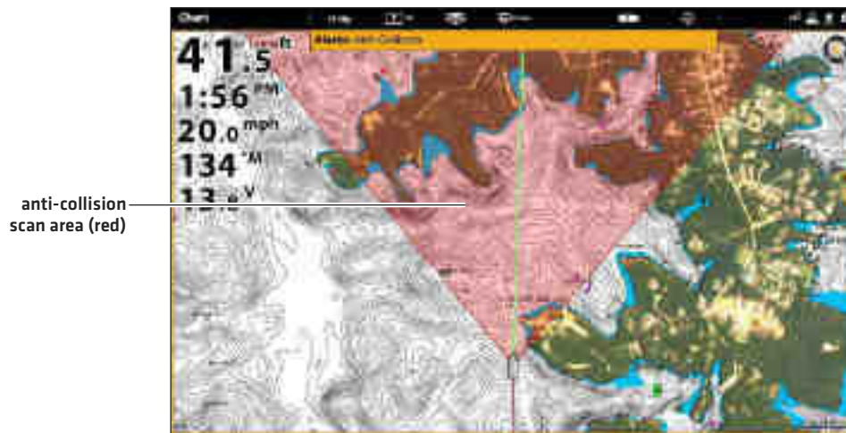
Chart View with Anti-Collision Overlay Turned On (Navionics)
