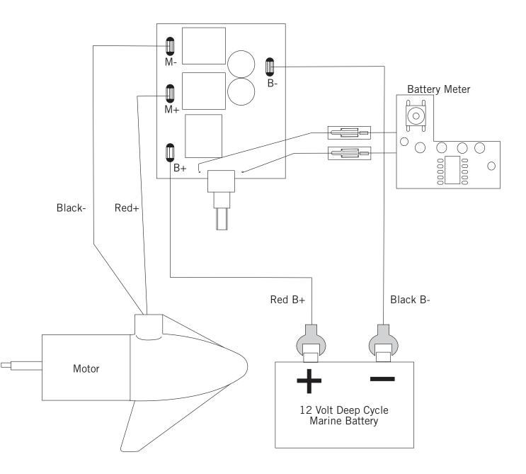
**NOTICE:** Double-check your motor's voltage for proper connections. Over-Current Protection Devices are not shown in this illustration.
