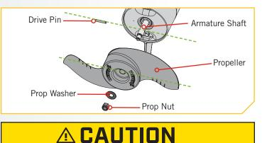
Disconnect the motor from the battery before beginning any prop work or maintenance.
