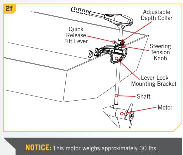
**NOTICE:** This motor weighs approximately 30 lbs. We recommend having a second person help with the installation.
